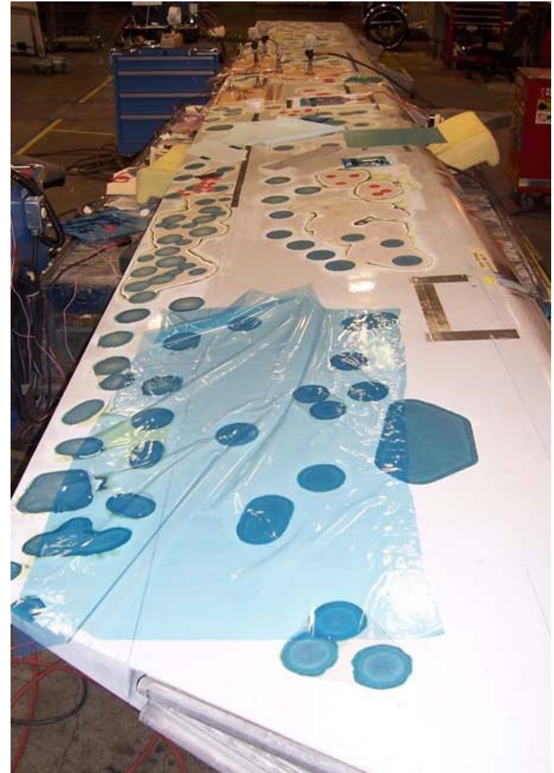
Outboard Elevator after hail
