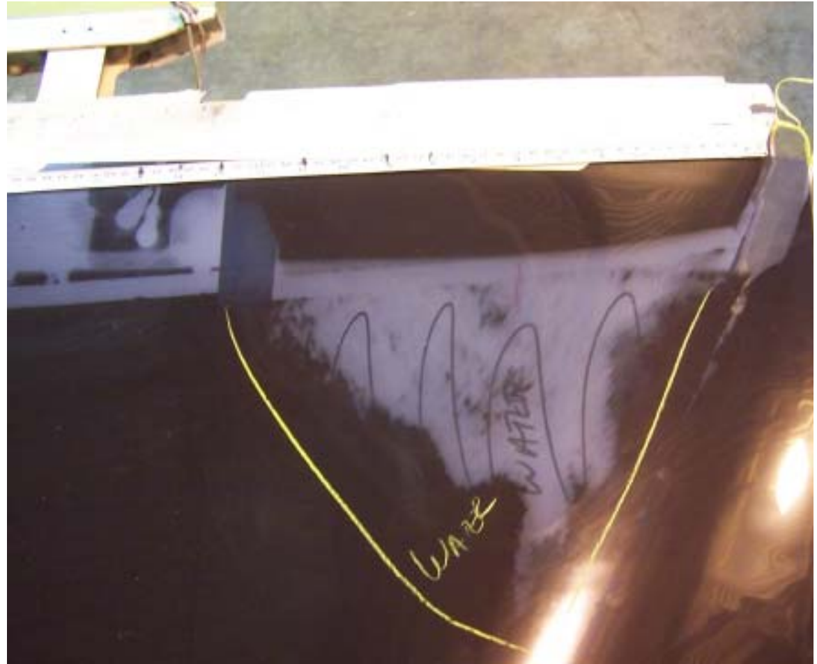
X-ray of outboard end of Aileron showing extent of water ingress into honeycomb
