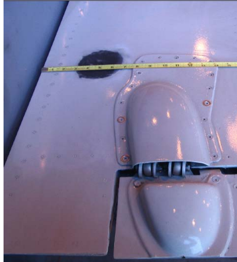
Elevator skin puncture in critical area
